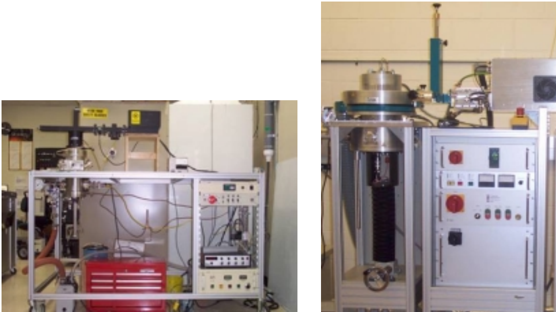
Figure 2.4: Two MPECVD systems at USF. (a) ASTeX; (b) IPLAS.
